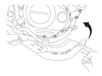
4. Attach  $6 \times 10$  mm socket bolts with washers to the front bracket (already attached). Tighten to  $10 \text{ N} \cdot \text{m}$ .
